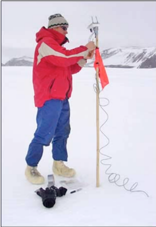
Bamboo is used for mounting, because it's lightweight and resilient to the Antarctic environment.
