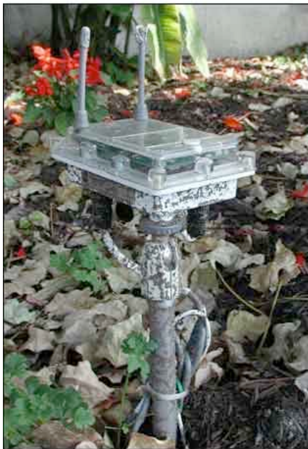
Sensor Web pod 15 at Huntington Botanical Gardens is covered in mud from nearby watering and has had an antenna chewed on by a small animal.
