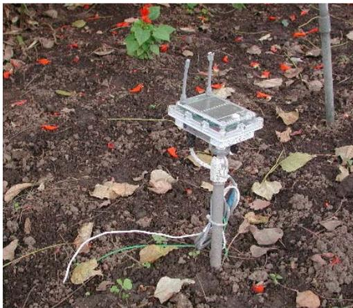
**Figure 5. Pod 15 at the Huntington Gardens. Note the right antenna is chewed. The two subterranean probes measure soil temperature and soil moisture.**
